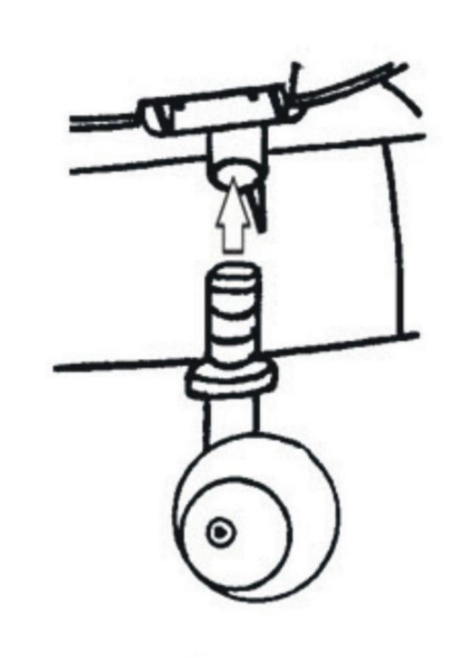
Insert the wheels into the moulded socket in the direction indicated by the arrow. Then push firmly until clicks into place.
