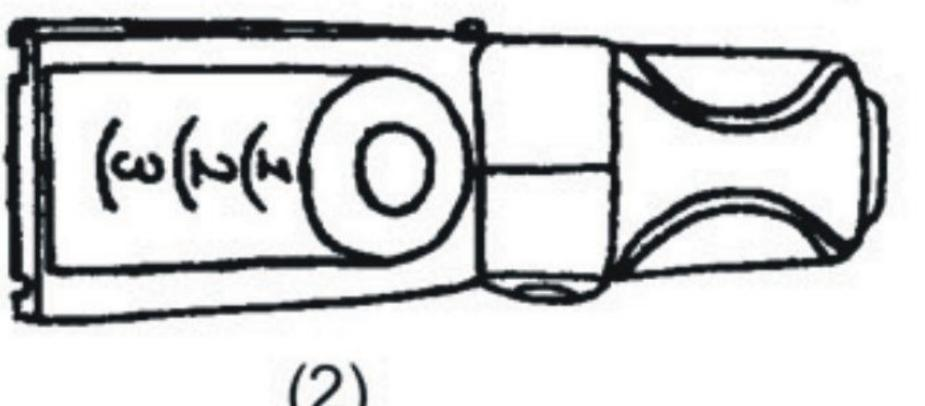
Turn one side of frame supporter outward (1) until you hear the frame supporter lock into position (2).
