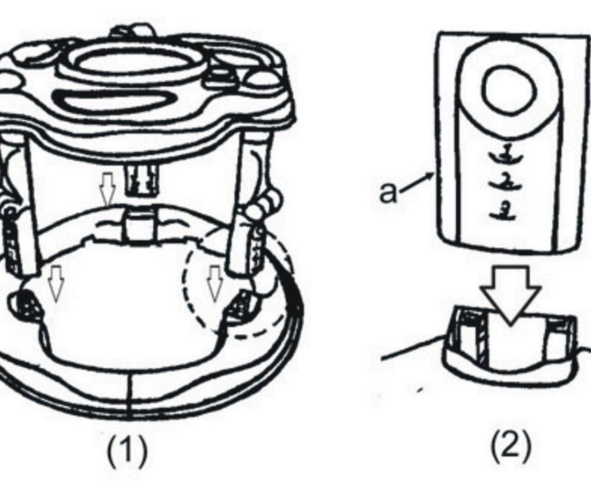
Place the base section of the jumperloo on the floor. Slot the end of frame supporters 'a' into the holes indicated in the drawing(1). Push the frame supporters into the base section. Ensure that the frame supporters are full inserted before proceeding.
