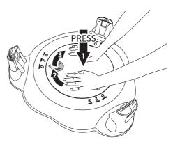
Push down and turn the platform move to either of the 2 options below.
