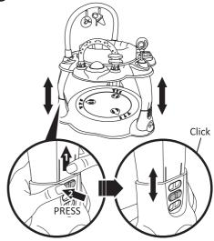
Use your thumb to press the button while bringing the leg up or down until you hear a click to adjust the height. There are 3 height adjustments.
