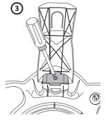
Screw on lid to secure the legs in place.
