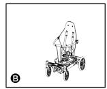
2. Hold down the chassis with one hand and lift the seat with the other hand to open up and erect the seat until it clicks into place. Figures C & D.
