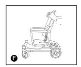
4. Push down the lever behind the seat to fold the seat forward. Figures G & H.
