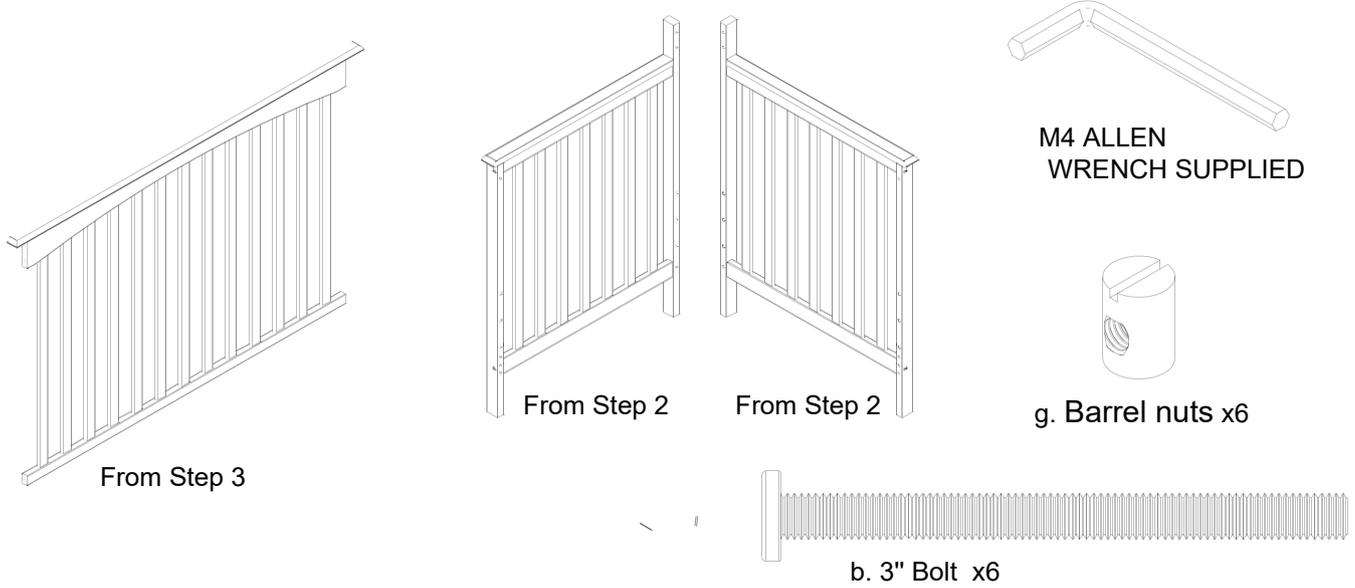
Attach step 2 to the assemblies from step 3 using (6) 3" Bolts (Part b) and (6) Barrel nuts (Part g). Tighten with the M4 Allen Wrench.
