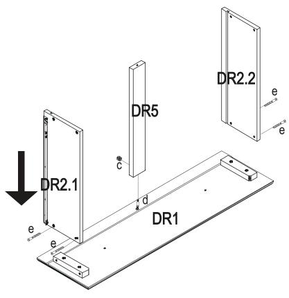
Connect drawer side panel (DR2) to front panel (DR1) by using 1" screw (e).
