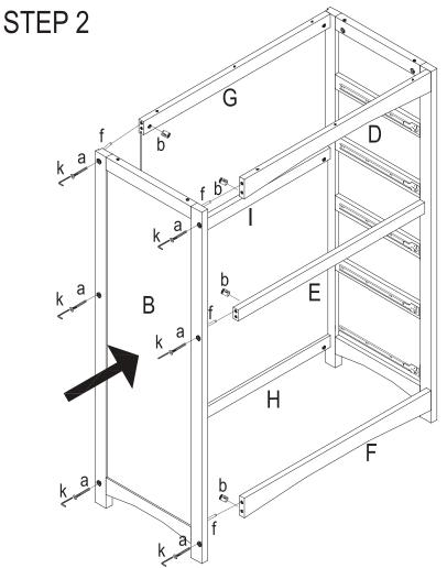
Assemble left panel (B) to the assembled parts use the same way as shown in STEP 1.
