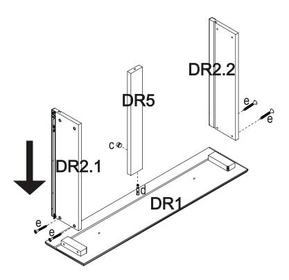
Connect side panel (DR2) to front panel (DR1) by using 1" screw (e).
