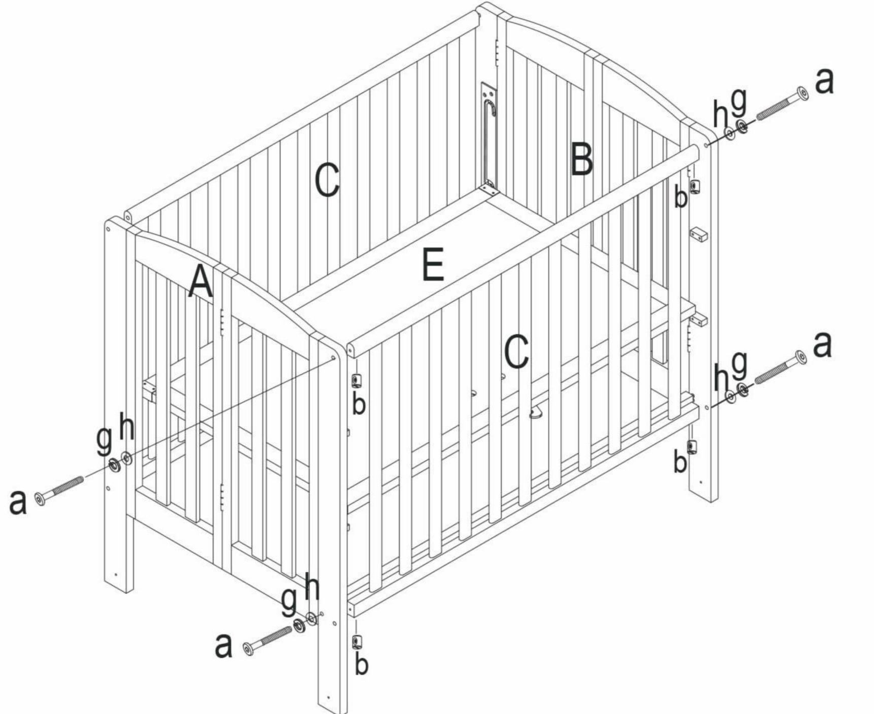
Connect rail (C) and stabilizer bar (D)to the headboard (A & B) by screws (a) and nuts (b), wood dowel (d), washer (g), washer (h). DO NOT fully tighten the bolts.
