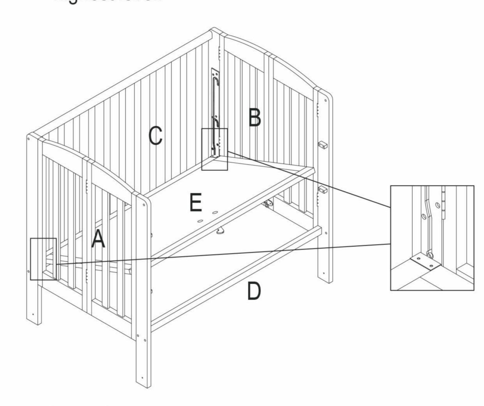
STEP 6 Select the desire level, and use both hand to lift up the mattress base, then adjust the level to your require height of the 3 level.
