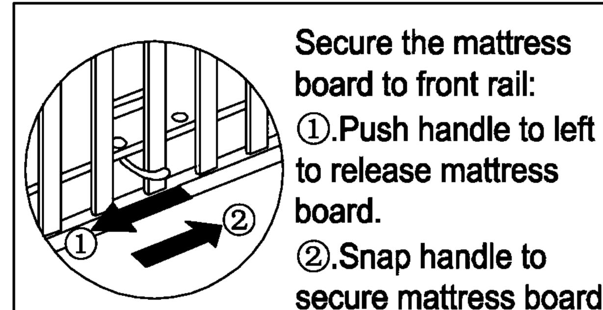
Secure the mattress board to front rail: 1).Push handle to left 2.Snap handle to
