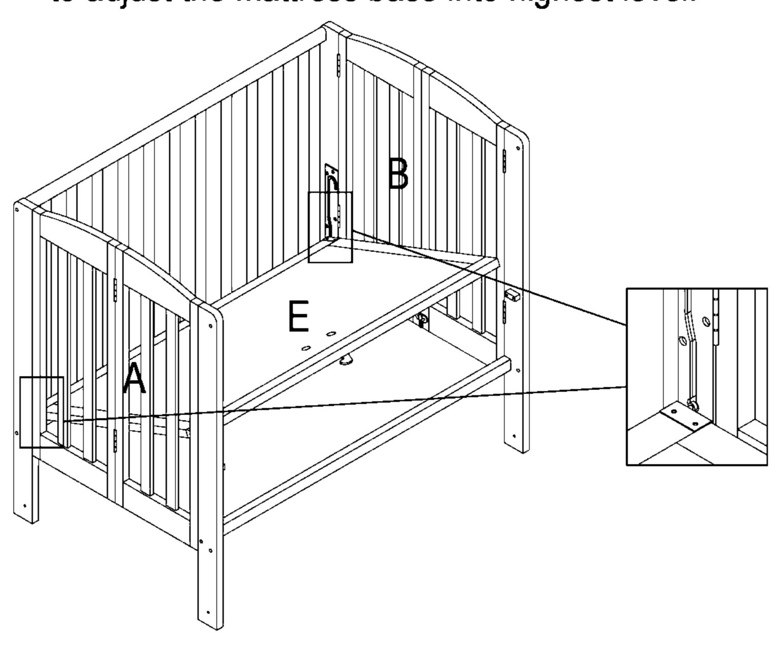
STEP 6 Select the desire level, and use both hand to lift up the mattress base, then adjust the level to your require height of the 2 level.
