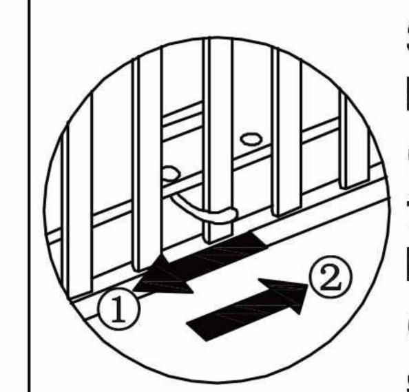
Secure the mattress board to front rail: ).Push handle to left to release mattress
