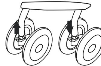
6. When the wheel fork is upturned, it can be runned with one direction otherwise, it can be renned around.
