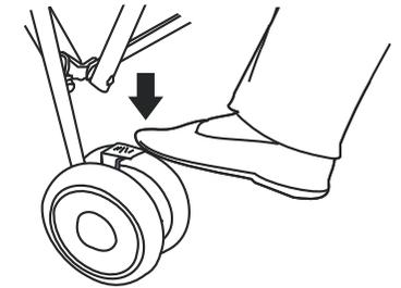
7. Step on the brake of the back wheels and lock the stroller.
