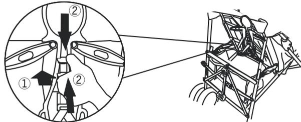
5. (1) Use the thumb to press the top plastic piece. (2) Use the forefinger to withstand plastic piece on the below and use two finger to adjust it.
