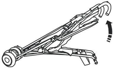
1. Release the red hook , hold the handle and pull upwards.
