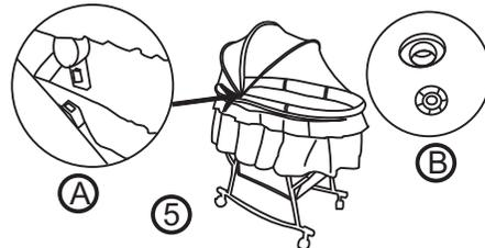
A. Insert the clip into the plastic on tube, to fix the mosquito net.
