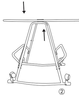
Joint the upper part to bottom part by 2 fastening bolts, secure all screws tightly by spanner before use.
