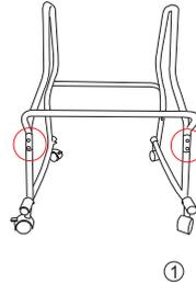
Connect the bottom tube to both sides by screws.
