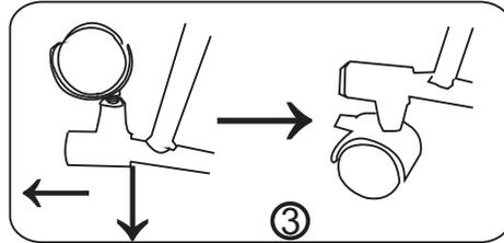
Put the wheels sideways and revolve the wheels to be on stand (as figures).
