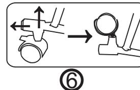
Put the wheels outwards and revolve the wheels be fixed, it can be rocked smoothly for baby.
